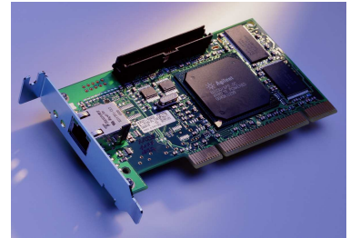
Agilent RMC Plus L 1.0 N2521A-AT1 Low-Profile PCI card 10/100 Base-T LAN port for alerting and remote access
